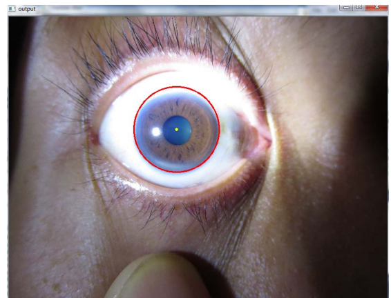
Fig 6. Hough Circle Transform Result
